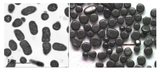
Fig. 2. Dusted gunpowder grains (on left), very heavily glazed gunpowder (on right)
