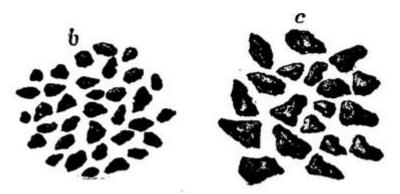
Fig. 1. Black powder grain flakes
