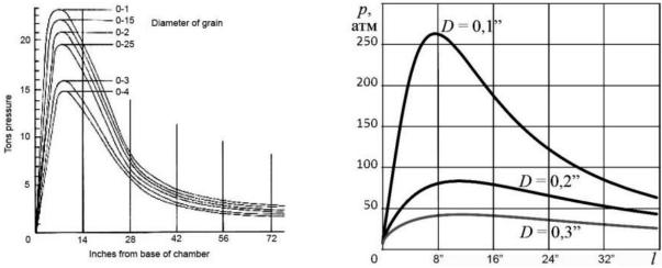
Fig. 3. Grain pressure curves (Mitiukov, Crawford, 2012)
