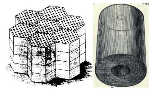
Fig. 4. Rodman full-bore perforated prismatic cake (on left), pellet 1 ¼ inch diameter (on right)
